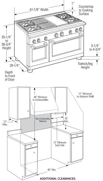
Allow 12" minimum clearance to an adjacent wall on each side.
